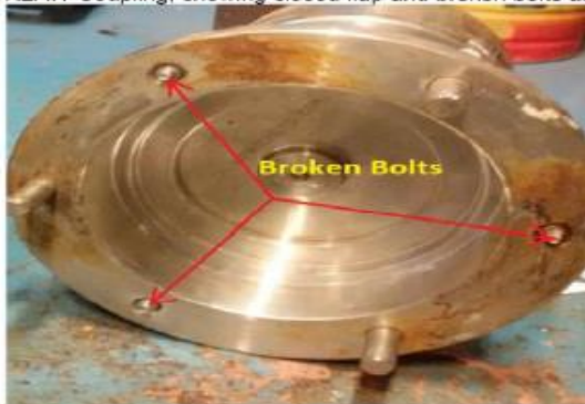
KLAW Coupling, showing closed flap and broken bolts after breaking away
