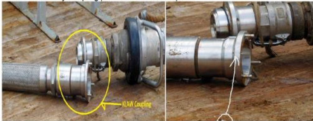
KLAW Break Away Coupling photos after it broke apart:
