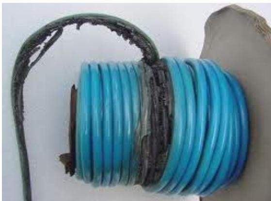
Example of Insulation breakdown resulting from heat accumulation.
