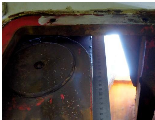
Picture of shark jaw mechanical link OUT of its over center position and position of proximity sensor when the shark jaw gave up (Green light is off)
