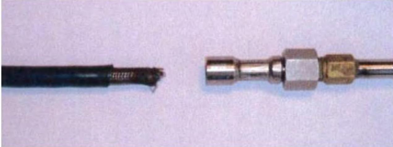
Following the review of an independent post-incident hose inspection report undertaken by the hose supplier, and analysis of historical data from previous accidents of this nature; it has been concluded that the primary cause of the blowback was due to “near adiabatic compression” occurring in the high pressure hose when the C/E quickly opened the cylinder valve against a closed regulator assembly valve.
