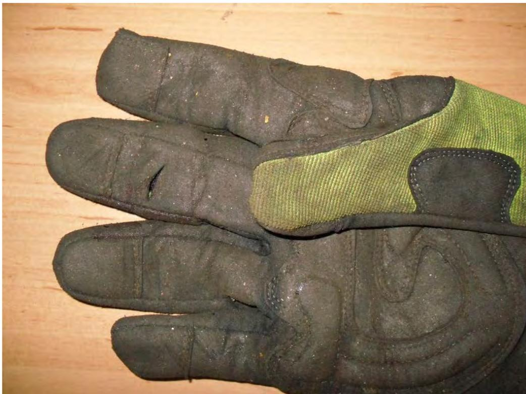
***Photo #1 – Glove in use showing cut inside middle finger***
