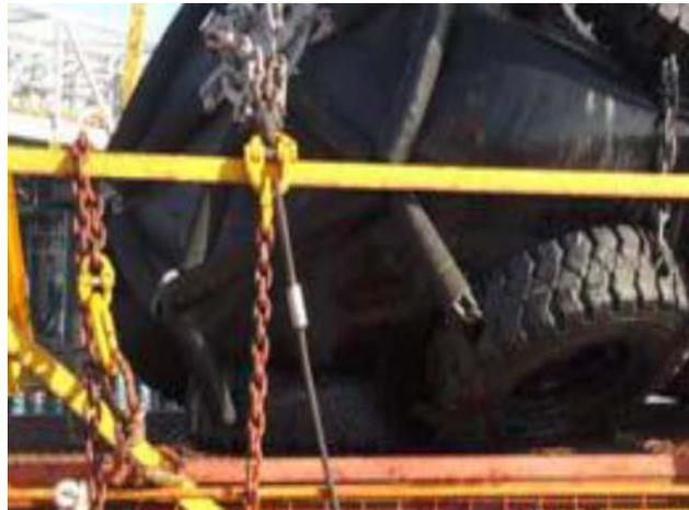
During the lifting of the 2nd fender, while the fender was between 2 and 5 metres above the holding cradle, the Superflex sling failed, causing the fender to fall, contacting a vertical post on the fender holder. The fender's structural integrity was compromised, causing the fender to deflate. The fender came to rest in the holding frame.
