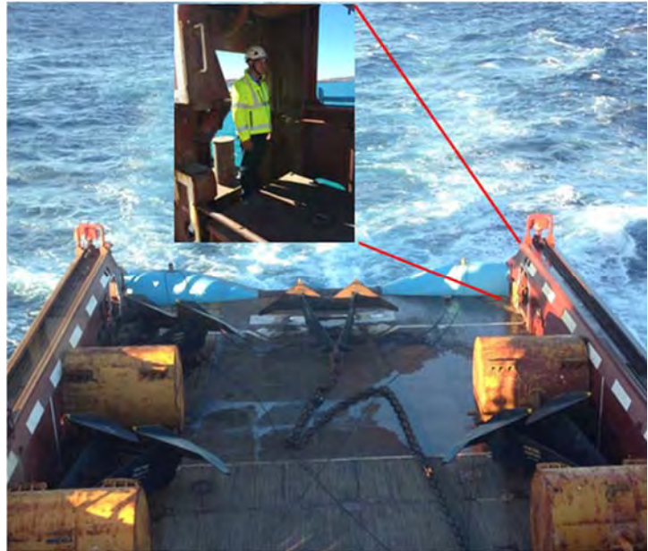
Worker position behind cargo barrier in area considered a 'safe haven'. Note: Configuration of equipment on vessel deck is not the same as when the incident occurred.
