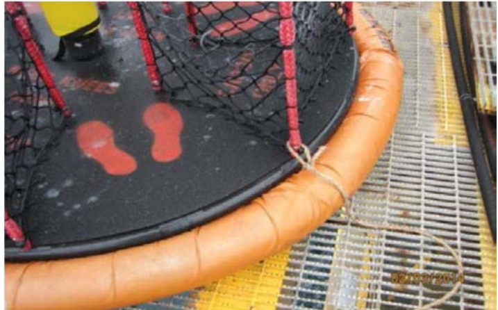
1/4" manila rope tag line that became entangled and wrapped around the riggers leg, causing him to be lifted 15' in the air
