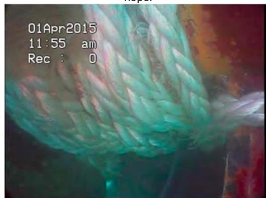
Picture depicting the mooring rope wrapped around the starboard propeller hub and the A Frame supporting the propeller shaft.
