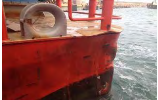
View of the damage sustained to Accommodation Barge due to contact with stern roller of AHT showing hull breach at deck level.
