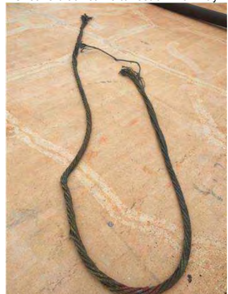
Failed Wire Grommet
