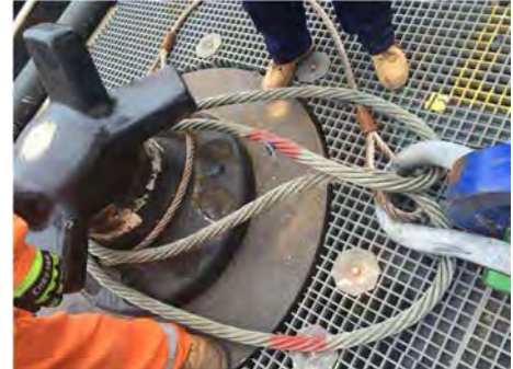
Safety Sling and Wire Grommet arrangement
