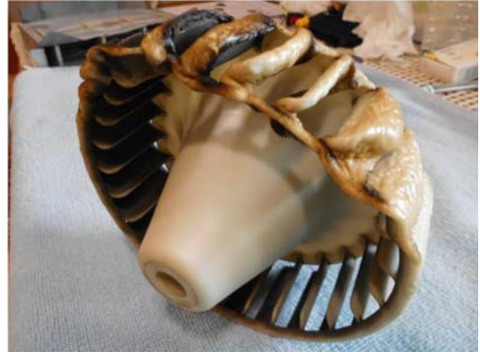
Damage to fan
