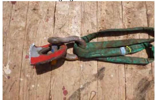
Damaged lifting lug
