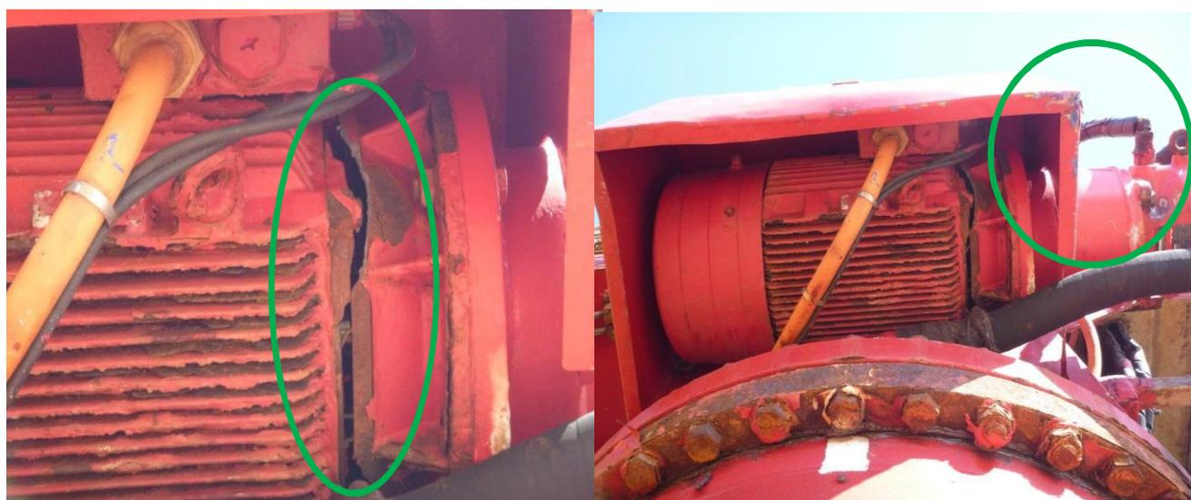
a) Close up of cracked motor.
